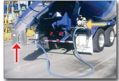
Figure 8. Chute washout bucket and pump
